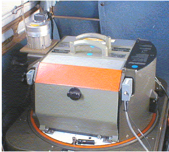
Figure 3: Leica RC20/30 Film Camera (Photo courtesy of Air Flight Service, Santa Clara CA)
